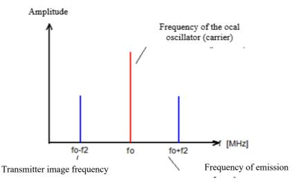
Figure 4. Spectral representation of the signal at the output of the mixer
