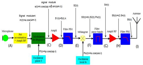
Figure 3. Detailed structure of the FM transmitter
